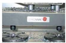
MTS chuck, able to automate. During the workpiece change, the contact surfaces are cleaned automatically.
