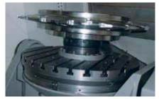
The Z-supports are placed as far on the outside that they provide a stable and precise support even for bigger workpieces.
