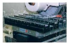
The UPC on the machine table constitutes the interface with the workpiece carrier. Resetting takes next to no time, and production can resume.
