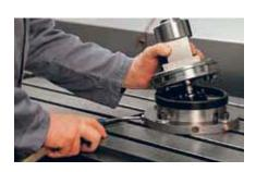
Clamped with  $\mu m$ -accuracy with one movement of the hand.
