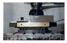
Low construction height leaves much room for workpieces.
