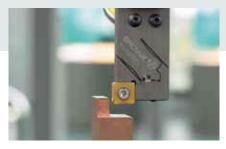
Simply ingenious: the 2D edge probe (EROWA patent) enables you to make the necessary measurements on radii, edges, corners and oblique surfaces.
