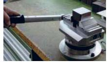
A few manual steps – and the workpiece is positioned in the Self Centering Vise.
