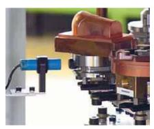
The EWIS<sup>TM</sup> Rapid identification system provides an overview of holders and pallets. With the modern transponder chips, every pallet can be identified at any time. The handling facilities examine the magazine loads automatically.
