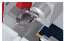
**Double gripper**Quick part change with the double gripper.
