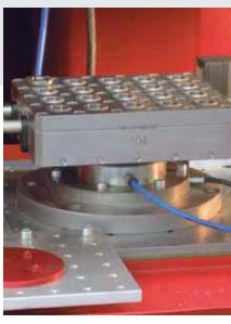
Fixture with set-up workpieces.
