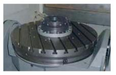
The existing attachment boreholes allow for quick mounting on all well-established machines.
