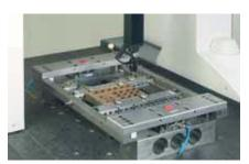
Presetting made easy. While the WEDM center is in operation, the next job is being preset quickly and accurately on the EROWA PreSet station.
