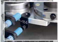
The EWIS<sup>TM</sup> Rapid identification system provides an overview of holders and pallets. With the modern transponder chips, every pallet can be identified at any time. The handling facilities examine the magazine loads automatically.
