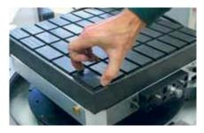
Thanks to the medium duct between chuck and pallet, workpieces may be clamped pneumatically, hydraulically or with a vacuum.
