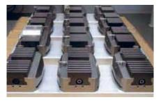
Flexible clamping devices. EROWA center clamps on MTS pallet.
