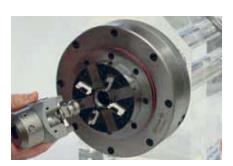
The ITS chuck is opened through the integrated air coupling.
