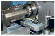
Horizontal chuck on a dividing head.
