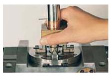
The workpiece is clamped with the precision of the ITS tooling system, with a repeatability of 0.002 mm.
