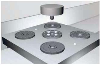
Several MTS chucks mounted on or directly integrated in the machine table.
